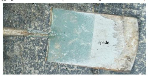
The shovel is great for digging holes in new ground. It's made to penetrate hard soil, letting all the gardener's weight rest on one point. It requires less force to break tough ground with a shovel than if you use a spade, just as one tap on a nail is more likely to sink it into wood than if you hammered on a razor blade.
